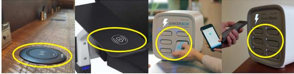
Fig. 5: Illustration of public wireless charging stations and power bank rental services. An attacker can maliciously compromise these facilities to use their coils to capture EM emanations.
